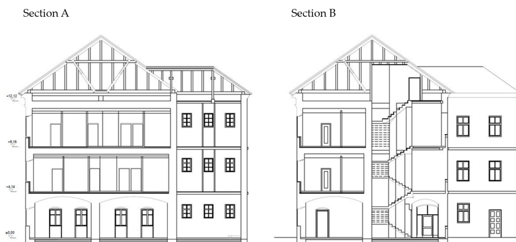
Figure 6. Transversal building sections A and B.
