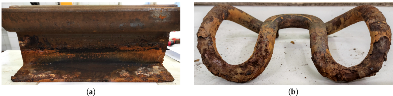
Figure 2. Exemplified condition of (a) rail sample and (b) fastening clip at the end of the laboratory corrosion test [28].
