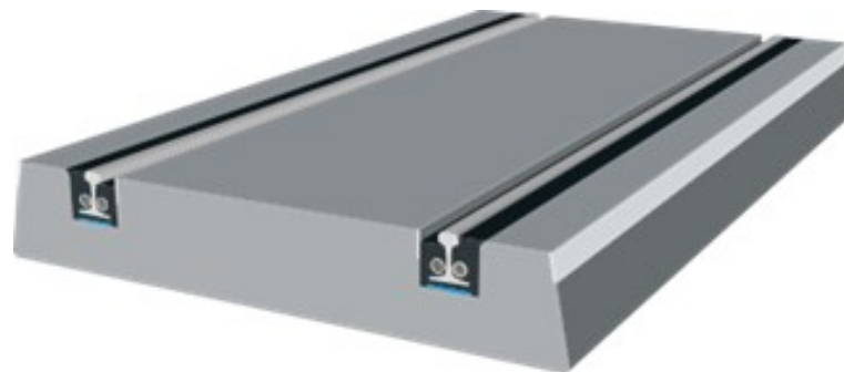
Figure 3. Track with continuously fastened rails [33].
