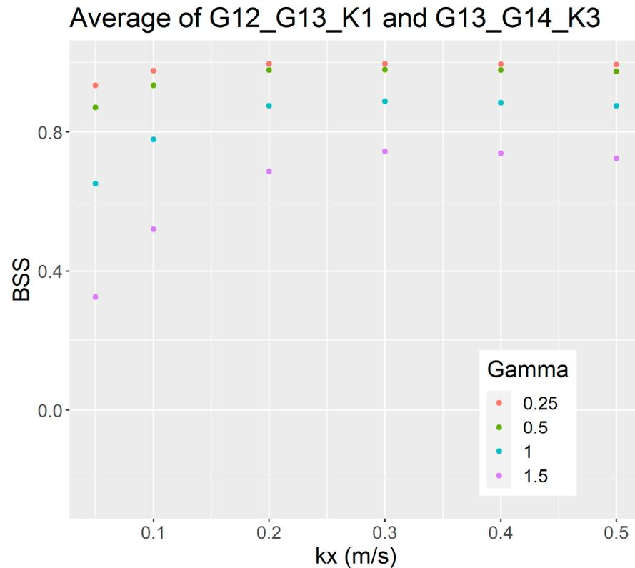
**Figure 7.** Average of Brier skill scores for wave events G12\_G13\_K1 and G13\_G14\_K3 for each combination of different hydraulic conductivity and transport coefficient values. Highest Brier skill score value (of 0.995) is obtained for the combination of hydraulic conductivity 0.3 m/s and transport coefficient 0.25.
