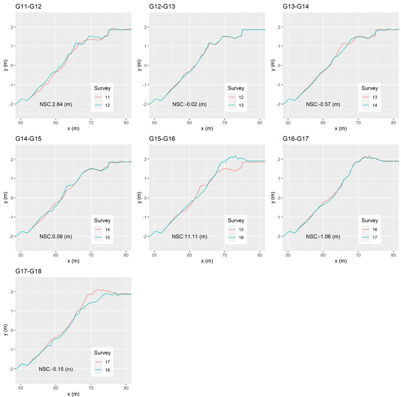
**Figure A2.** Change in profile sediment distribution for Profile 1 after each geodetic survey 11–18. NSC is short for net sediment change and is calculated by subtracting the earlier from the later survey and summing all values. Only three sets of surveys (G12–G13, G13–G14, and G14–G15) have net sediment change less than 1 m.
