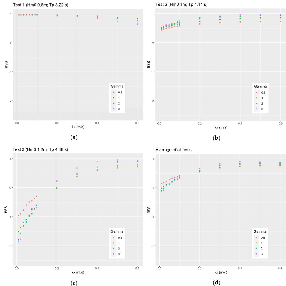
**Figure 4.** Relationship between hydraulic conductivity (kx), Brier skill score, and transport coefficient (gamma) for (a) Test 1, (b) Test 2, and (c) Test 3, and for (d) the averaged Brier skill score for all three tests.
