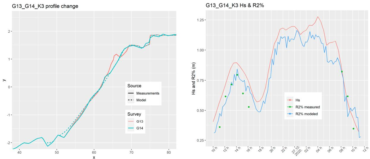
**Figure 9.** Simulation of G13\_G14\_K3 wave event results: changes in sediment profile (left) and wave runup during the event (right). Profile change shows crest buildup, which the model correctly predicts (dashed and solid cyan). Modeled (blue line) and measured (green dot) wave runup are in agreement and are less than the measured significant wave height (red line).
