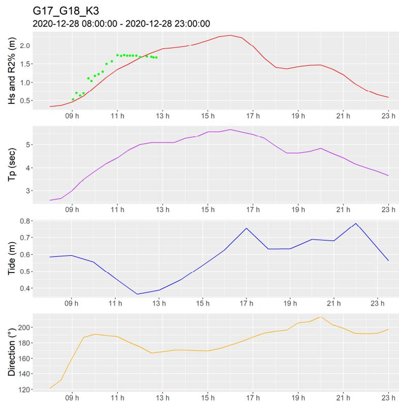
**Figure 3.** Parameters of wave event G17\_G18\_K3 used to simulate the event using XBeach-Gravel: significant wave height (Hs, red line) and 2% exceedance rate of wave runup (R2%, green dots); peak period (Tp, purple line); mean sea level change (blue line), and wave direction (yellow line).
