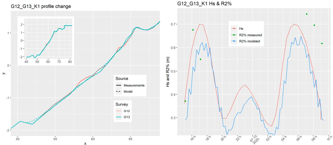
**Figure 8.** Simulation of G12\_G13\_K1 wave event results: changes in sediment profile (left) and wave runup during the event (right). No major sediment change occurred on the profile; simulated wave runup (blue line) follows the significant wave height (red line) while measured runup (blue dots) is slightly underpredicted.
