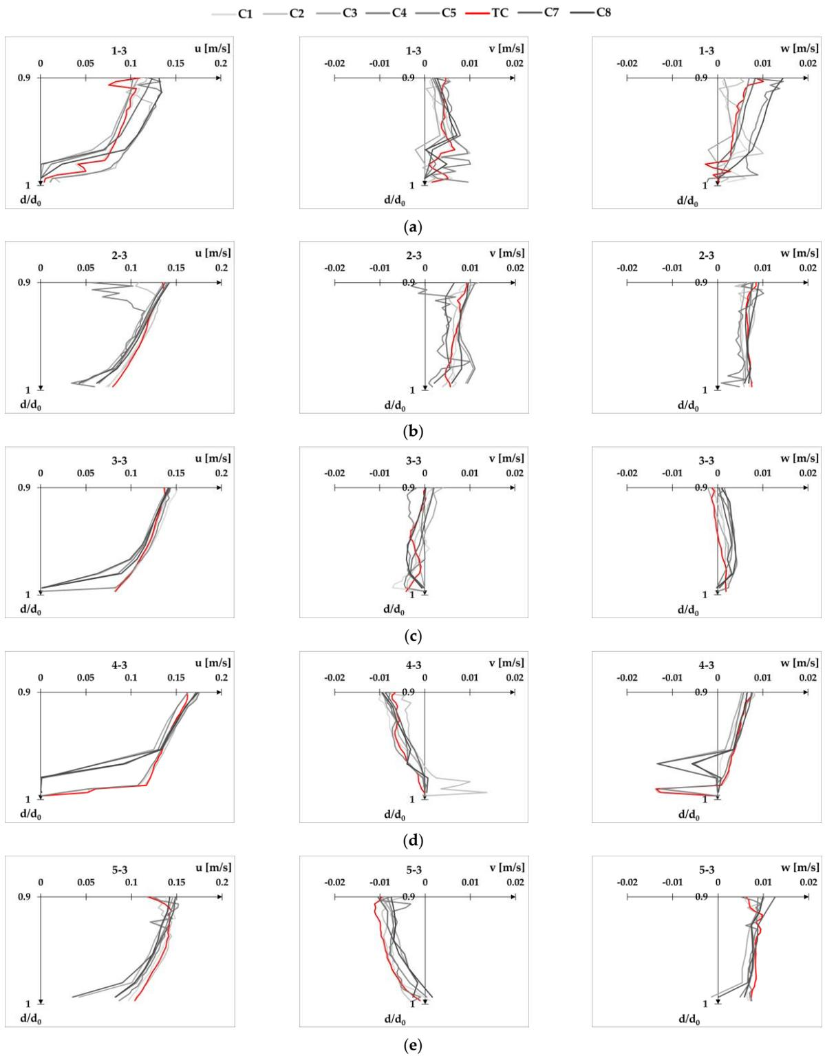
**Figure A6.** Velocity profiles for flow condition Q1d1 at XS-DS plotted separately for each velocity component  $u$ ,  $v$ , and  $w$ : point 1-3 (a), point 2-3 (b), point 3-3 (c), point 4-3 (d), and point 5-3 (e).
