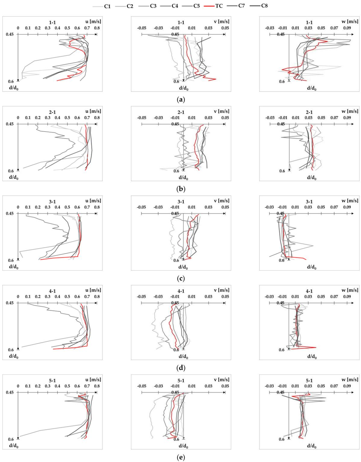
**Figure A19.** Velocity profiles for flow condition Q2d2 at XS-DS plotted separately for each velocity component  $u$ ,  $v$ , and  $w$ : point 1-1 (a), point 2-1 (b), point 3-1 (c), point 4-1 (d), and point 5-1 (e).
