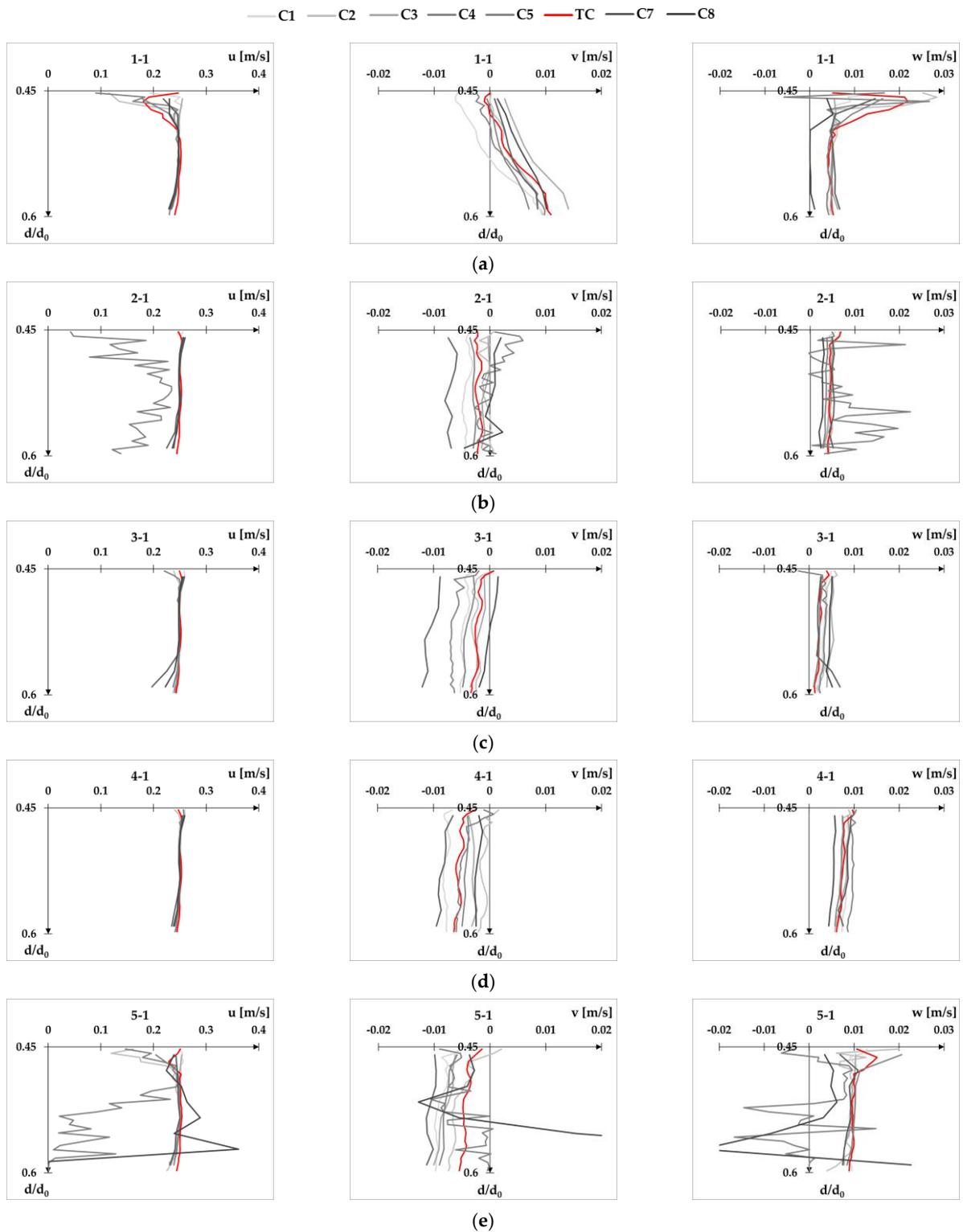
**Figure A7.** Velocity profiles for flow condition Q1d2 at XS-US plotted separately for each velocity component  $u$ ,  $v$ , and  $w$ : point 1-1 (a), point 2-1 (b), point 3-1 (c), point 4-1 (d), and point 5-1 (e).
