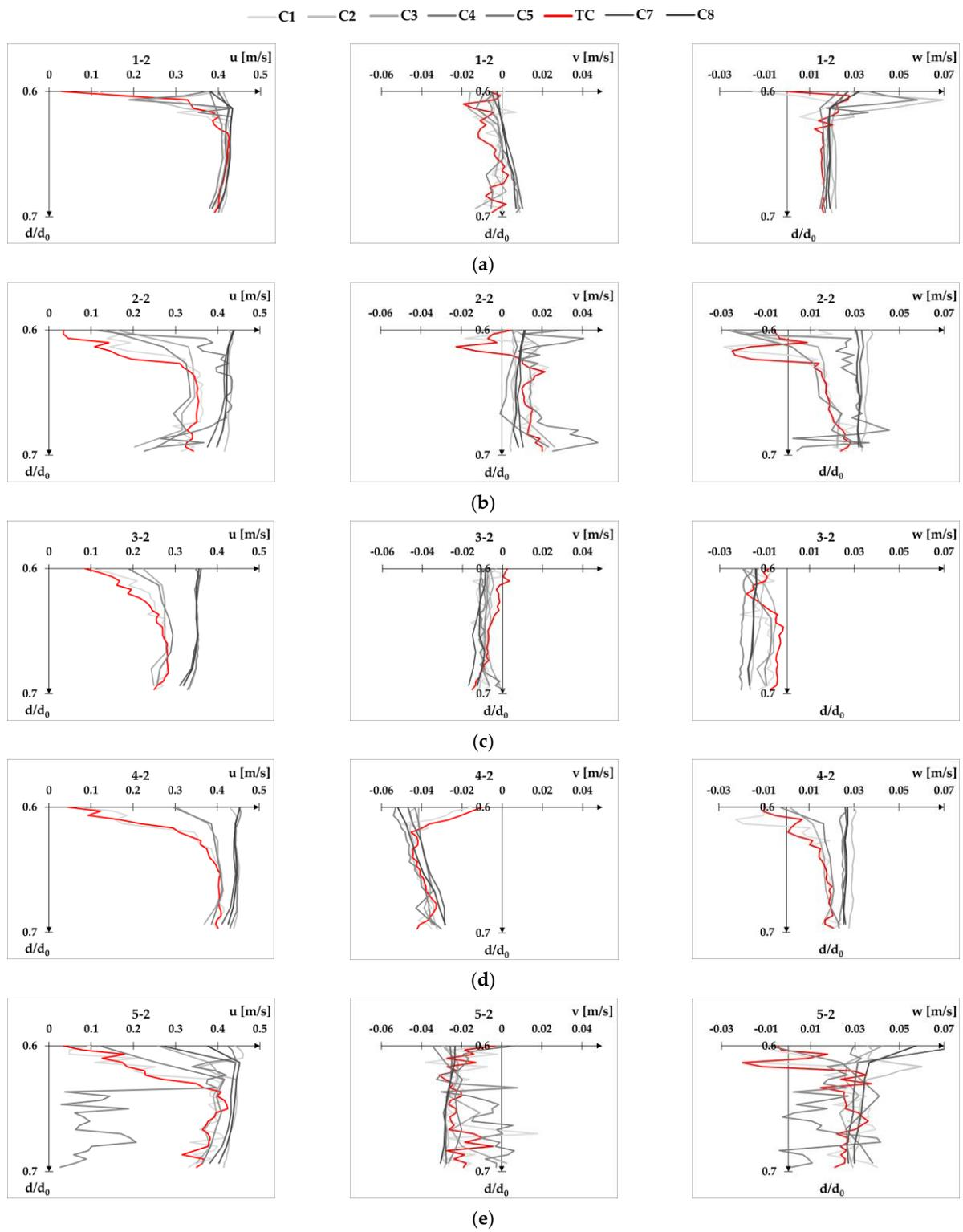
**Figure A15.** Velocity profiles for flow condition Q2d1 at XS-DS plotted separately for each velocity component  $u$ ,  $v$ , and  $w$ : point 1-2 (a), point 2-2 (b), point 3-2 (c), point 4-2 (d), and point 5-2 (e).
