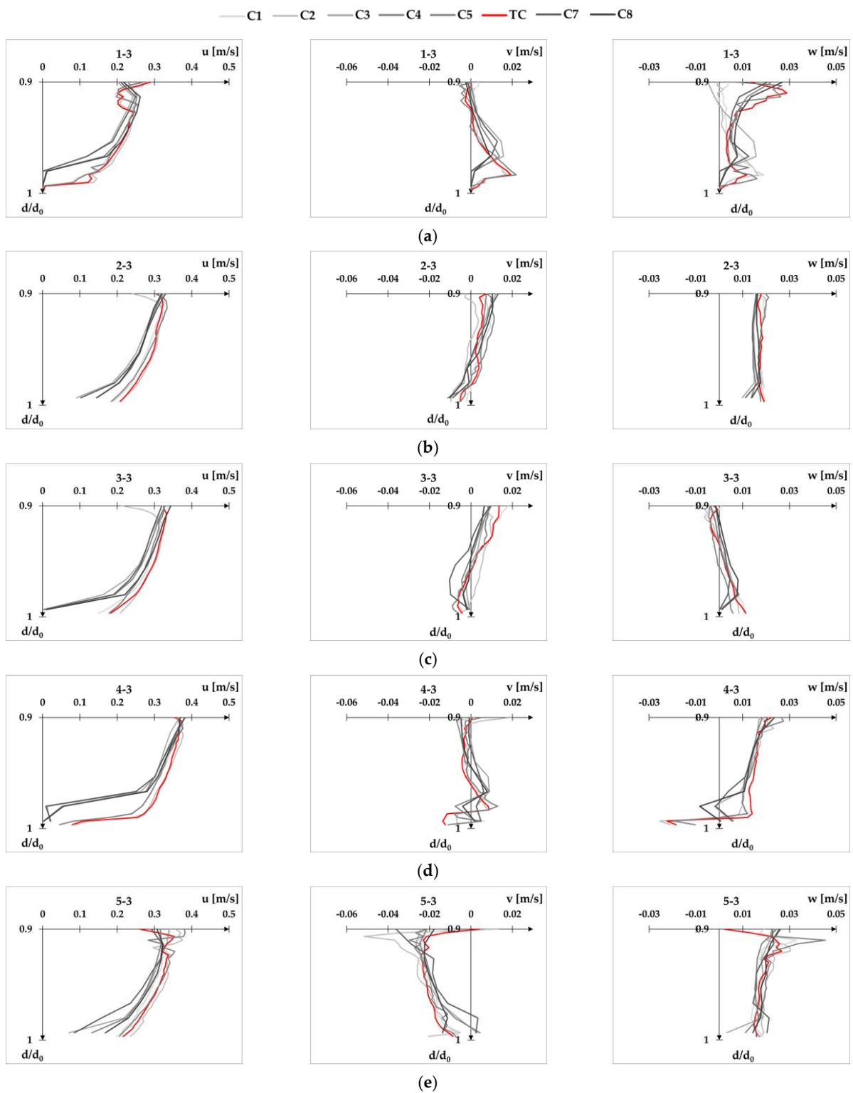
**Figure A16.** Velocity profiles for flow condition Q2d1 at XS-DS plotted separately for each velocity component  $u$ ,  $v$ , and  $w$ : point 1-3 (a), point 2-3 (b), point 3-3 (c), point 4-3 (d), and point 5-3 (e).
