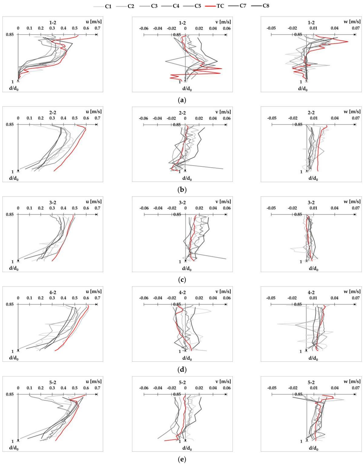
**Figure A20.** Velocity profiles for flow condition Q2d2 at XS-DS plotted separately for each velocity component  $u$ ,  $v$ , and  $w$ : point 1-2 (a), point 2-2 (b), point 3-2 (c), point 4-2 (d), and point 5-2 (e).
