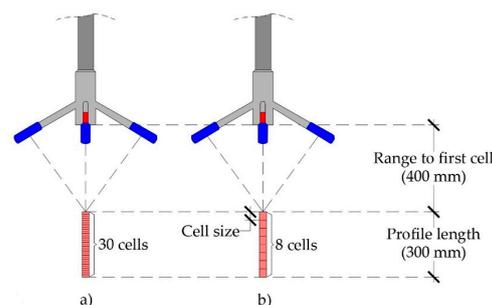
**Figure 4.** Spatial distribution of the measurement cells of the ADVP with different CS: CS = 1 mm (a), CS = 4 mm (b).
