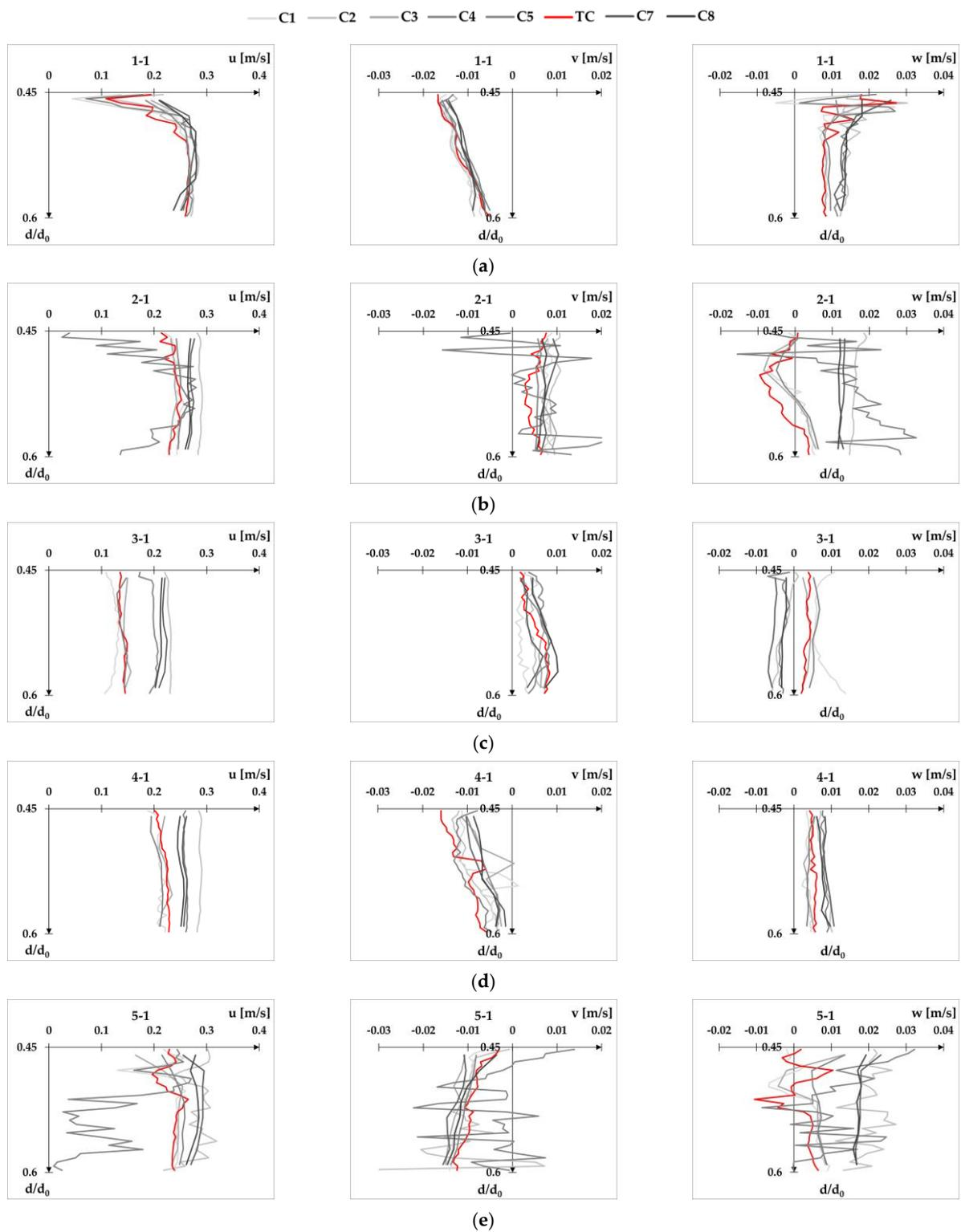
**Figure A9.** Velocity profiles for flow condition Q1d2 at XS-DS plotted separately for each velocity component  $u$ ,  $v$ , and  $w$ : point 1-1 (a), point 2-1 (b), point 3-1 (c), point 4-1 (d), and point 5-1 (e).
