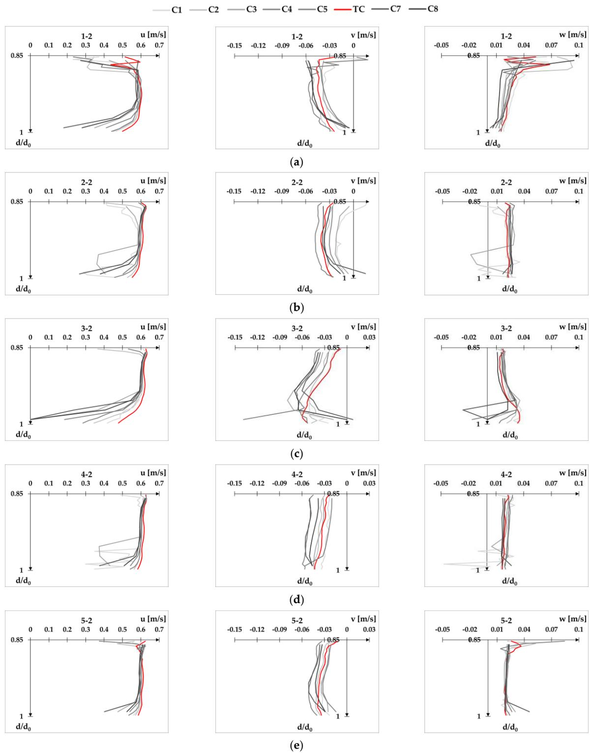
**Figure A18.** Velocity profiles for flow condition Q2d2 at XS-US plotted separately for each velocity component  $u$ ,  $v$ , and  $w$ : point 1-2 (a), point 2-2 (b), point 3-2 (c), point 4-2 (d), and point 5-2 (e).
