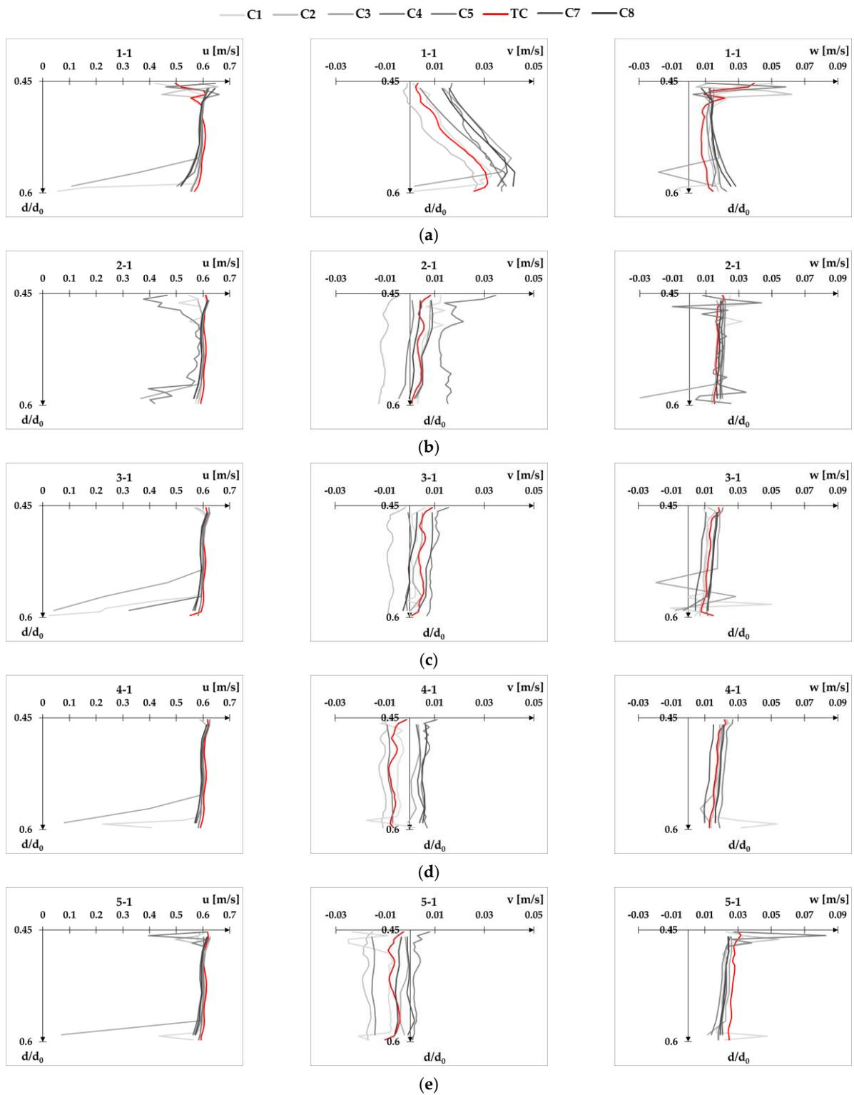
**Figure A17.** Velocity profiles for flow condition Q2d2 at XS-US plotted separately for each velocity component  $u$ ,  $v$ , and  $w$ : point 1-1 (a), point 2-1 (b), point 3-1 (c), point 4-1 (d), and point 5-1 (e).
