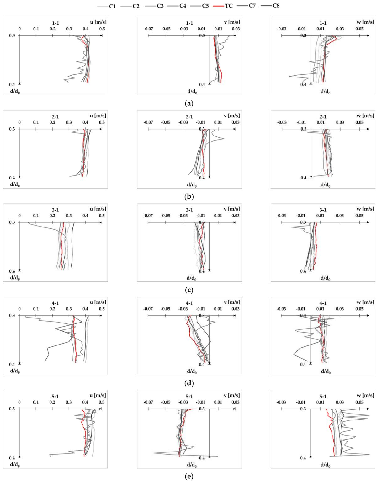
**Figure A14.** Velocity profiles for flow condition Q2d1 at XS-DS plotted separately for each velocity component  $u$ ,  $v$ , and  $w$ : point 1-1 (a), point 2-1 (b), point 3-1 (c), point 4-1 (d), and point 5-1 (e).
