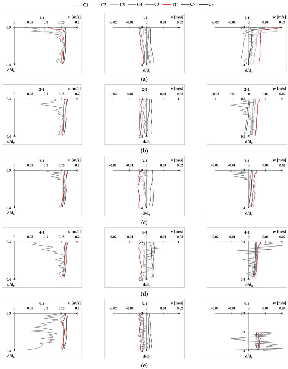
**Figure A1.** Velocity profiles for flow condition Q1d1 at XS-US plotted separately for each velocity component  $u$ ,  $v$ , and  $w$ : point 1-1 (a), point 2-1 (b), point 3-1 (c), point 4-1 (d), and point 5-1 (e).
