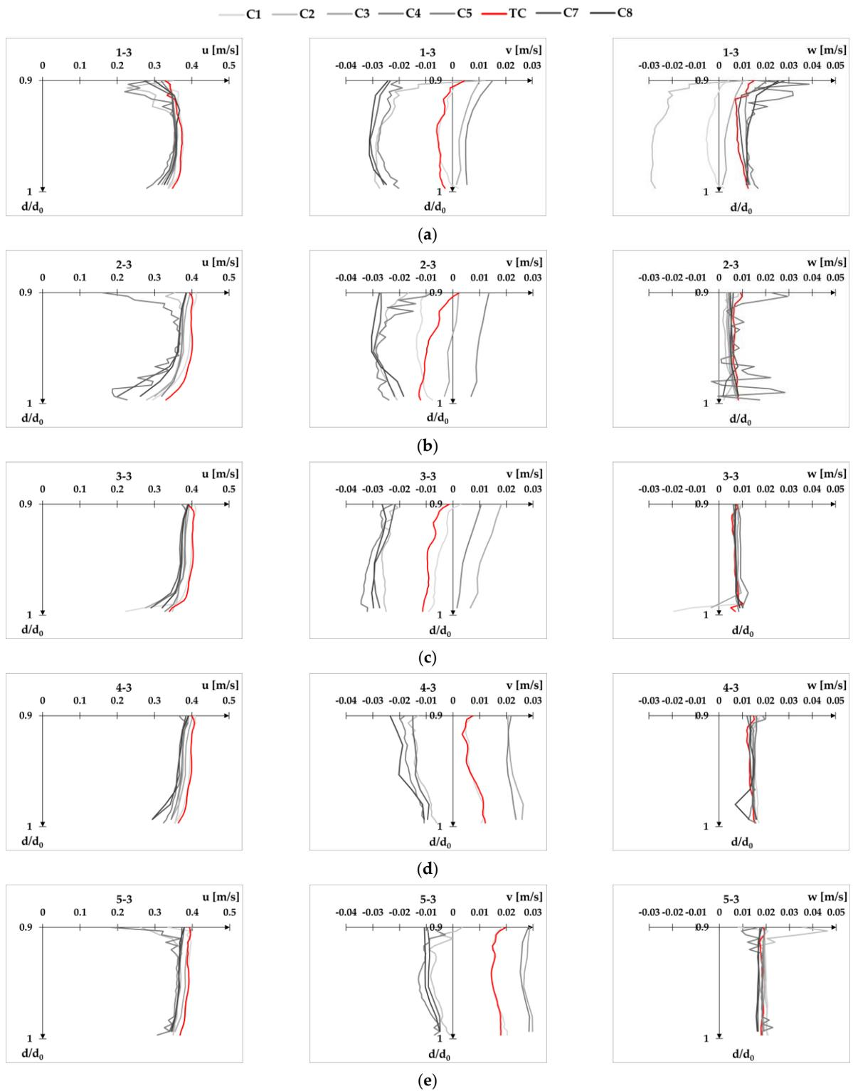
**Figure A13.** Velocity profiles for flow condition Q2d1 at XS-US plotted separately for each velocity component  $u$ ,  $v$ , and  $w$ : point 1-3 (a), point 2-3 (b), point 3-3 (c), point 4-3 (d), and point 5-3 (e).
