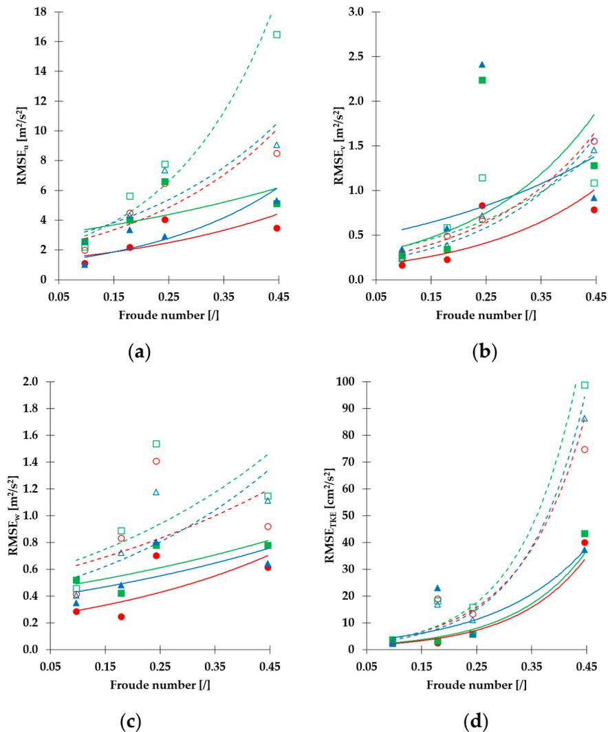
**Figure 14.** Change in RMSE with Froude number: velocity component  $u$  (a), velocity component  $v$  (b), velocity component  $w$  (c), and TKE (d). Solid and dotted lines represent trendlines for XS-US and XS-DS, respectively.
