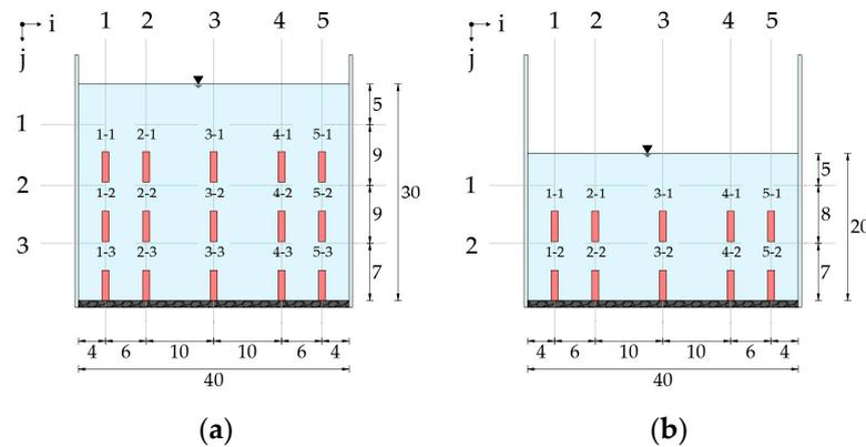
**Figure 3.** Scheme of the raster of the measurement points for a single experimental cross-section: layout for flow depth  $d_1 = 30 \text{ cm}$  (a), and layout for flow depth  $d_2 = 20 \text{ cm}$  (b); all lengths are given in centimeters.
