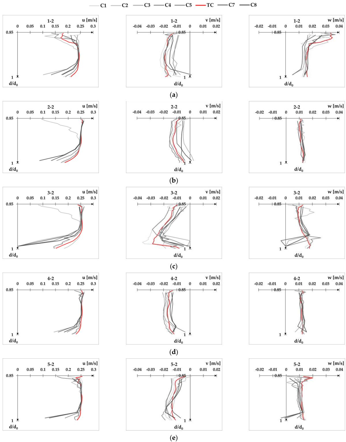
**Figure A8.** Velocity profiles for flow condition Q1d2 at XS-US plotted separately for each velocity component  $u$ ,  $v$ , and  $w$ : point 1-2 (a), point 2-2 (b), point 3-2 (c), point 4-2 (d), and point 5-2 (e).
