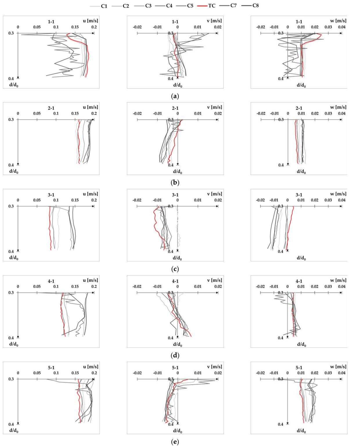
**Figure A4.** Velocity profiles for flow condition Q1d1 at XS-DS plotted separately for each velocity component  $u$ ,  $v$ , and  $w$ : point 1-1 (a), point 2-1 (b), point 3-1 (c), point 4-1 (d), and point 5-1 (e).
