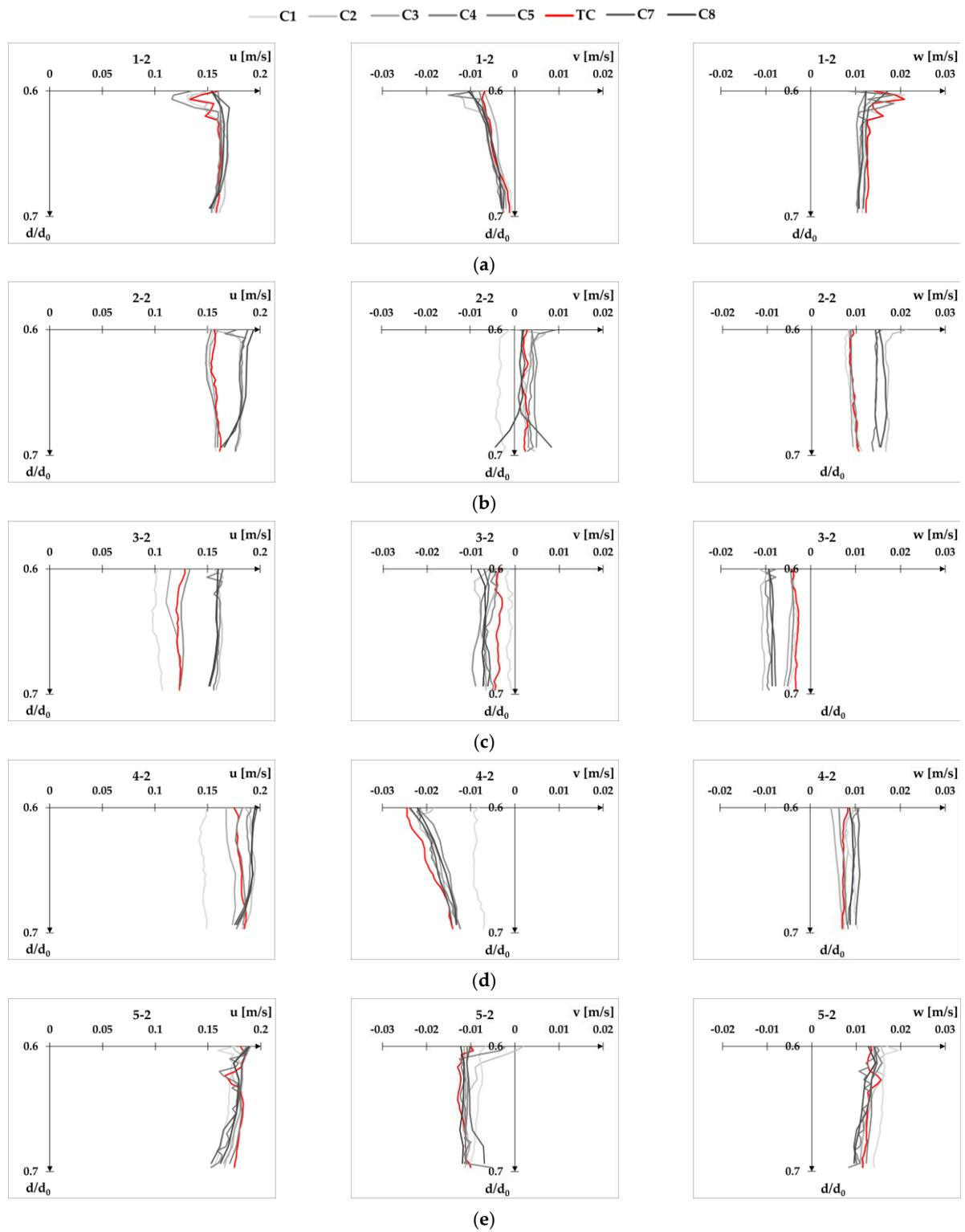
**Figure A5.** Velocity profiles for flow condition Q1d1 at XS-DS plotted separately for each velocity component  $u$ ,  $v$ , and  $w$ : point 1-2 (a), point 2-2 (b), point 3-2 (c), point 4-2 (d), and point 5-2 (e).
