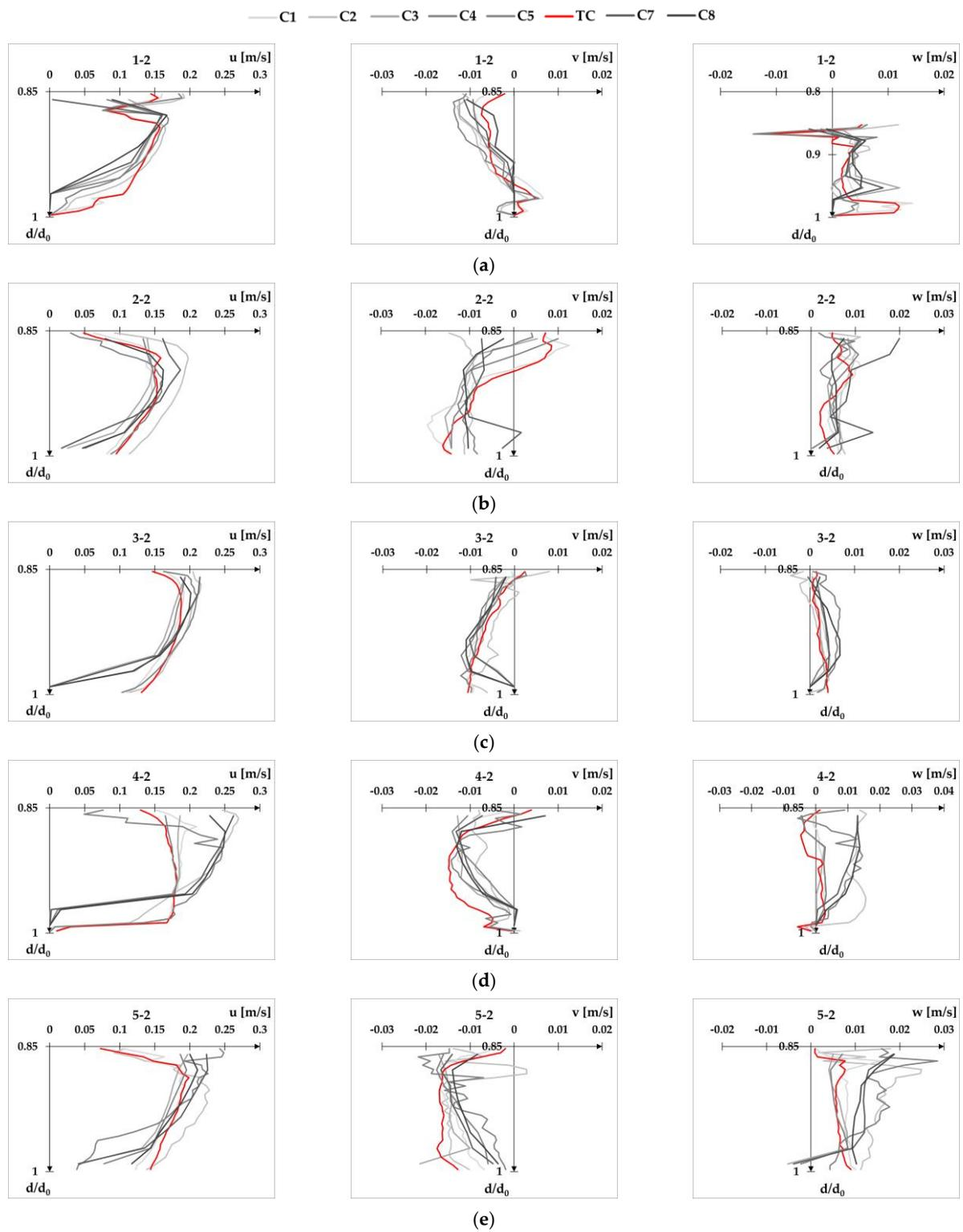
**Figure A10.** Velocity profiles for flow condition Q1d2 at XS-DS plotted separately for each velocity component  $u$ ,  $v$ , and  $w$ : point 1-2 (a), point 2-2 (b), point 3-2 (c), point 4-2 (d), and point 5-2 (e).
