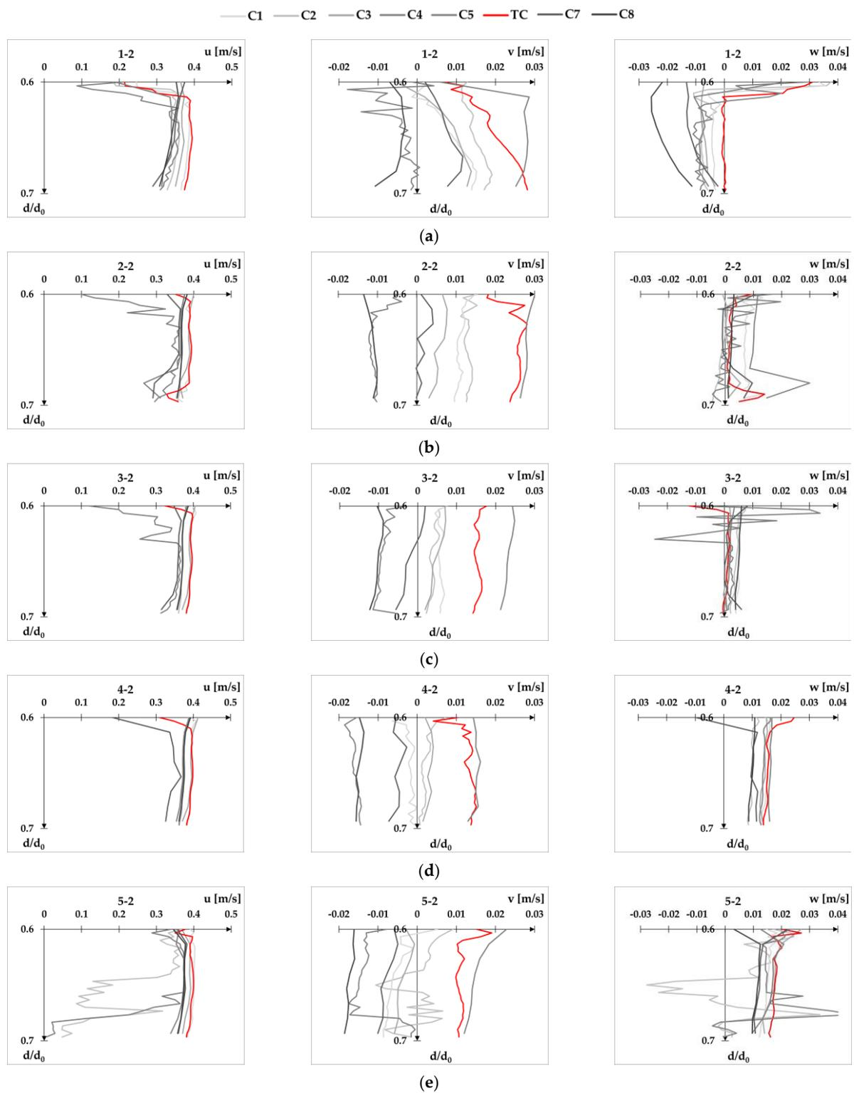
**Figure A12.** Velocity profiles for flow condition Q2d1 at XS-US plotted separately for each velocity component  $u$ ,  $v$ , and  $w$ : point 1-2 (a), point 2-2 (b), point 3-2 (c), point 4-2 (d), and point 5-2 (e).
