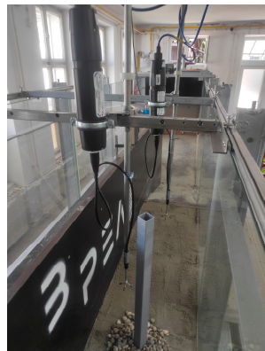
Figure 1. Photo of ADVP mounted on a cart for the hydraulic flume setup.
