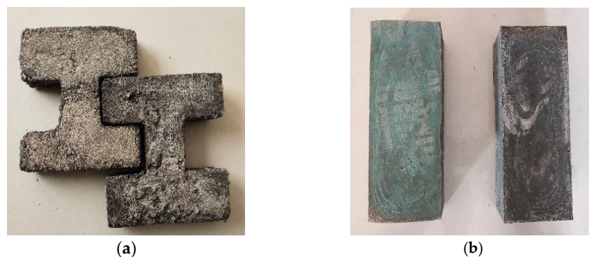
Figure 4. Waste plastic road paver blocks. (a) I-Shape Road Paver Block. (b) Waste plastic brick.
