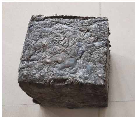
Figure 2. Size of the cube = 150 × 150 × 150 mm.
