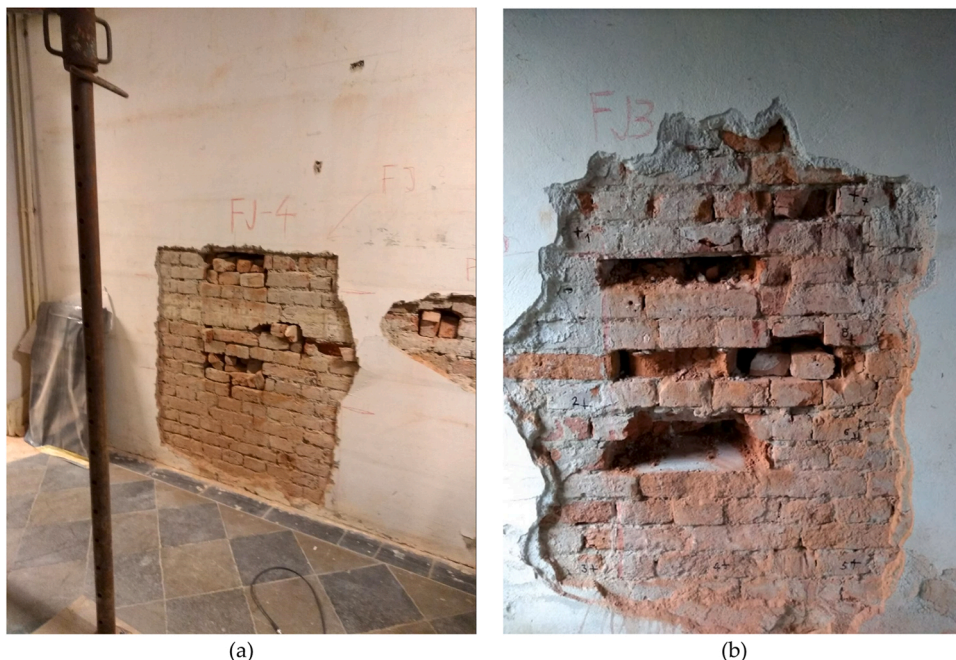
Fig. 5. Sonic tests were carried out at the same location of flat-jack tests: (a) Museum of Arts and Crafts; (b) Zagreb cathedral.
