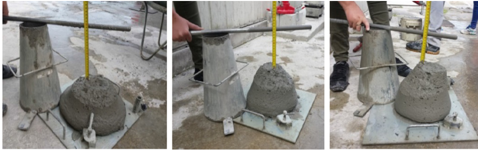
Fig. 6. Slump test for concrete with air entrainment: (a) without fibers, (b) with 0.9 kg/m 3 of RTPF, and (c) with 1.8 kg/m 3 of RTPF.
