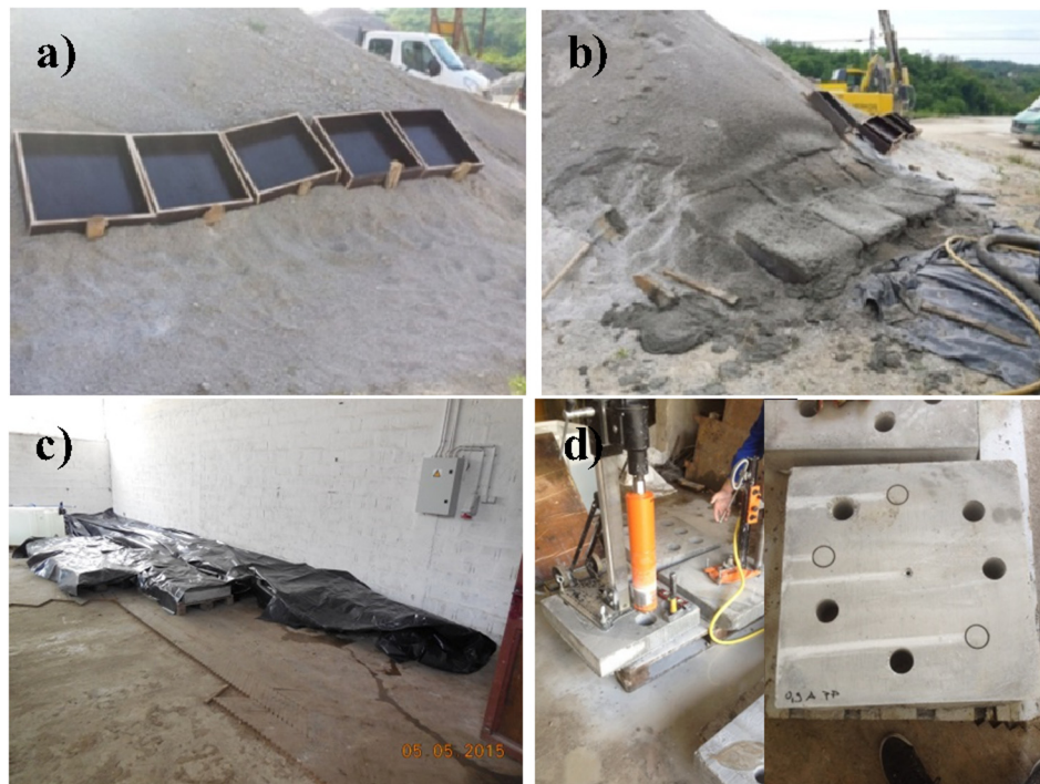
Fig. 5. Preparation of in-situ specimens: (a) molds, (b) specimens after spraying, (c) curing the panels (d) extraction of cores from panels.
