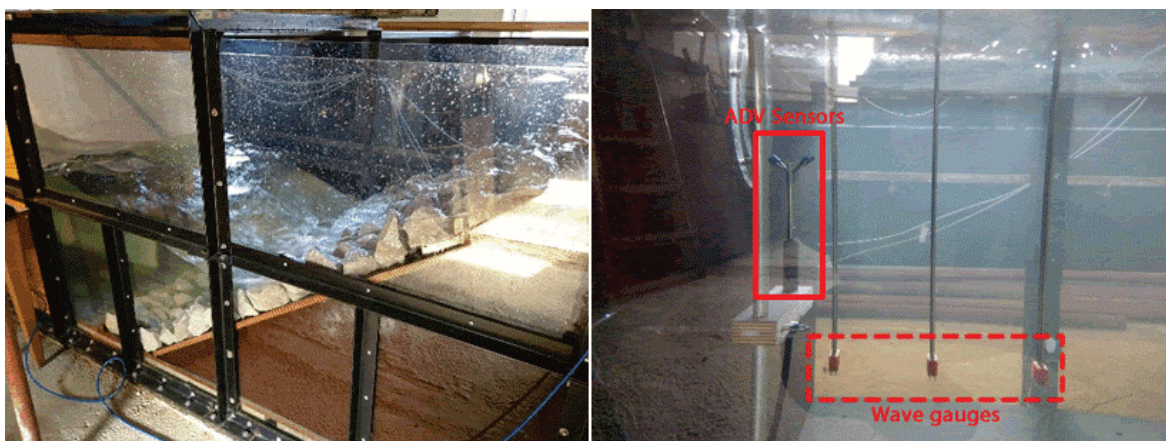
Figure 11 Waves at physical model of breakwater in the wave flume (left); ADV device behind the model of breakwater (right)
