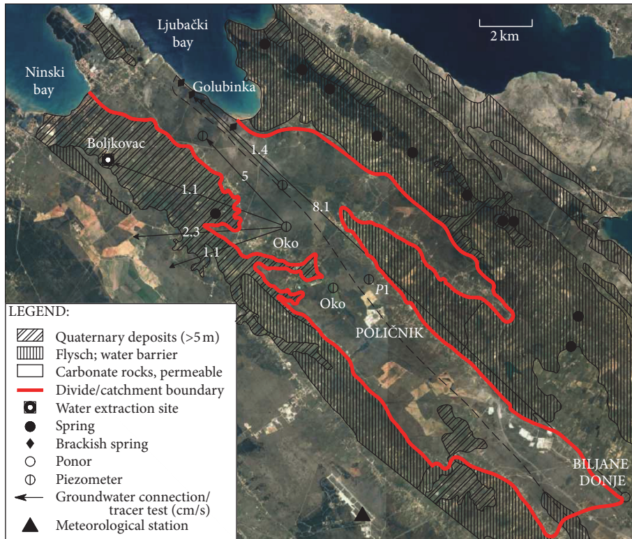
FIGURE 1: Schematic hydrogeological map of the Golubinka spring catchment area.
