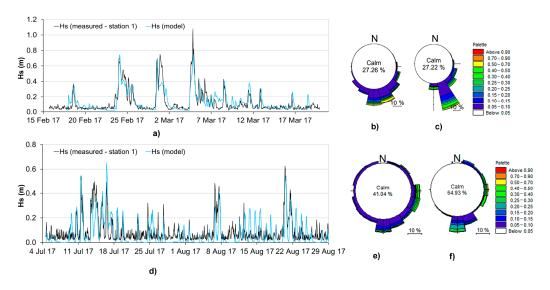
**Figure 19.** Comparison of measured and modelled time series of significant wave heights  $H_S$  at measurement station 1 for the (a) winter and (d) summer measurement periods with corresponding wave roses from (b,e) measured and (c,f) modelled data.
