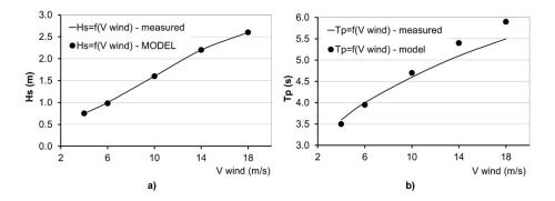
**Figure 18.** Relationship of measured and modelled (a) significant wave heights  $H_S$  and (b) peak period  $T_P$  against measured wind speed  $V_{wind}$ , under the action of wind from SSE direction in the course of 12 h (recording obtained from measurement at wave rider site in front of the main breakwater in Rijeka Harbour).
