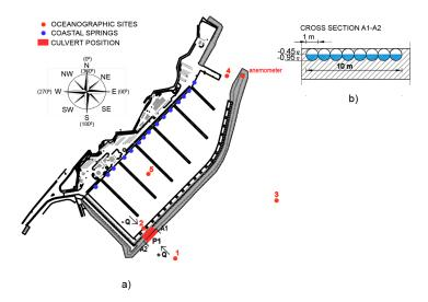
**Figure 3.** (a) Plan view of the oceanographic sites in the marina (ADCP 1–5—sea current and surface elevation measurements, ADCP 1, 2—wave parameters measurements, 2—PCM and CTD device, 1–5 vertical temperature and salinity profile), the coastal spring positions, the culvert position P1 and; (b) cross sections through the flushing culverts.
