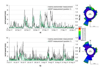
**Figure 5.** Time series of wind velocities and significant wave heights (measured at position 1, hourly averaged) with the corresponding wind rose for the (a) winter and (b) summer measurement periods.
