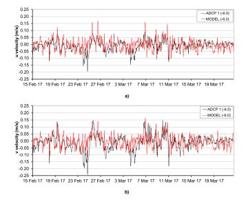
**Figure 10.** Comparison of measured and modeled hourly averaged (**a**) u velocity component and (**b**) v velocity component at a depth of -6 m at the position of ADCP 1 for the winter period.
