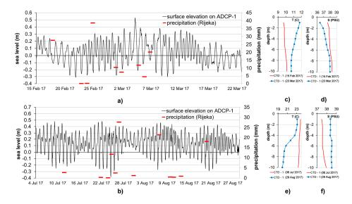
**Figure 4.** Time series of surface elevations recorded at the ADCP station 1 and daily precipitation at the meteorological station Rijeka ( $\phi = 45020'$ ,  $\lambda = 14027'$ ) for the (**a**) winter and (**b**) summer measurement periods; the sea temperature (T) and salinity (S) throughout the vertical sea column at site 1 for (C, **d**) the winter and (C, C) summer measurement periods.
