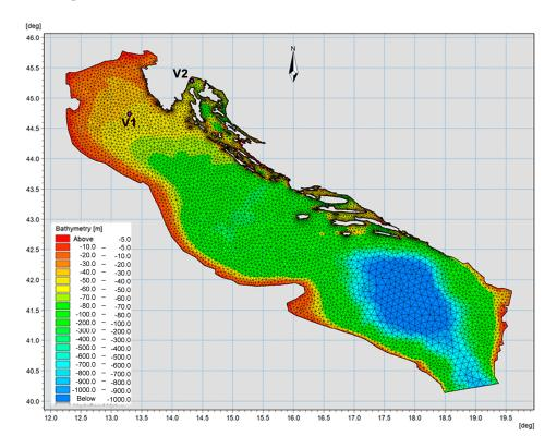
**Figure 16.** Model domain spatial discretization with unstructured finite volume grid on bathymetric background and locations of wave rider stations V1 ( $\phi = 44^{\circ}44.57'$  N,  $\lambda = 13^{\circ}17.98'$  E) and V2 ( $\phi = 45^{\circ}19.37'$  N,  $\lambda = 14^{\circ}18.7'$  E).
