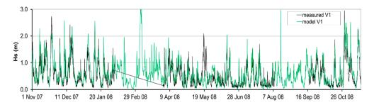
**Figure 17.** Comparison of measured and modelled time series of significant wave heights Hs at wave measurement station V1 in the northern Adriatic open-sea area ( $\phi = 44^{\circ}44.57'$  N,  $\lambda = 13^{\circ}17.98'$  E).
