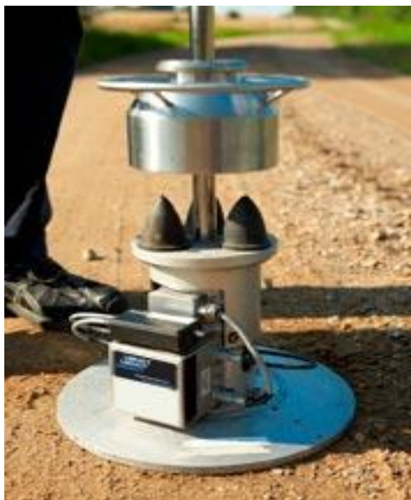
Slika 22 Prima 100 (preuzeto s https://www.impact-test.co.uk/products/5472-prima-100-portable-falling-weight-deflectometer/ )
